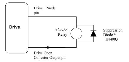
\*The suppression diode is critical for any open collector transistorized output when driving an inductive device such as a relay or electromechanical counter. Without this *"flyback diode"*, the open collector output can be permanently damaged. <u>Note</u>: External diode required with Mentor II & Quantum III only.
